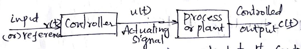
Reference input  $r(t)$  is applied to the controller which generates the actuating signal  $u(t)$  required to control the process which is to be controlled. process gives the desired controlled output  $c(t)$ .
